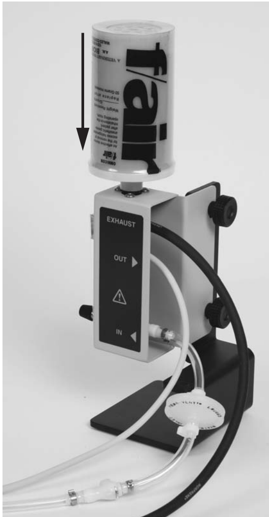
Figure 1-6. The included charcoal filter or a user-supplied charcoal filter presses onto the external output port on the docking station rotameter.
